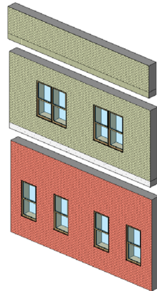
Exploded view of precast panelized wall system for area detailed at left.
